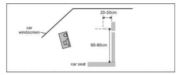
Figure E.2: Test Configuration for Vehicle mounted hands-free, receiving characteristics, with discrete measurement microphone
