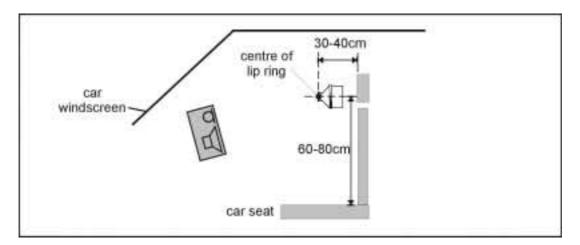
Figure E.3: Test Configuration for Vehicle mounted hands-free, sending characteristics, with discrete P. 51 artificial mouth
