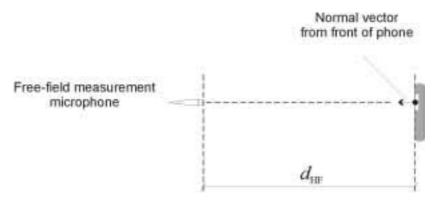
Figure E.5: Configuration of Hand-Held Hands-free MS, free-field microphone for receiving measurements
