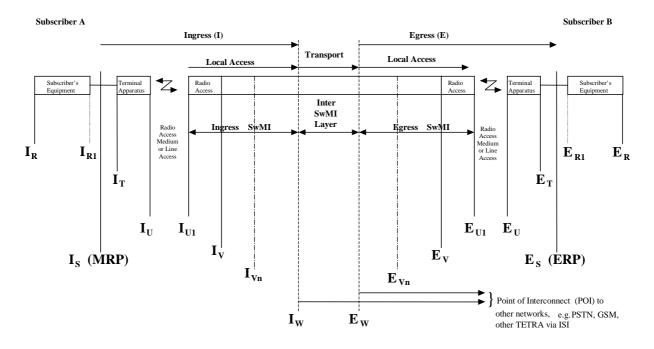
Figure 1: Intermediate Monitoring Point (IMP) model
