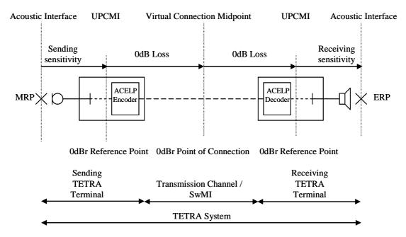
Figure 2: 0dBr points in a simplex connection
