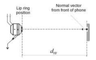
Figure E.6: Configuration of Hand-Held Hands-free MS, discrete P. 51 artificial mouth for sending measurements
