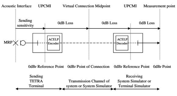
Figure 3: General access to terminals in a simplex connection
